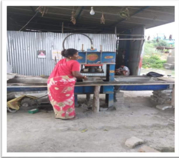
Gummidipoondi Block – M-Sand- utilization Production of Platform stones
